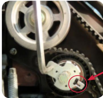
9. At the '3 o'clock position', turn the tensioner in the direction of the arrow (anti-clockwise), until the pointer is in the centre of the adjusting plate.
