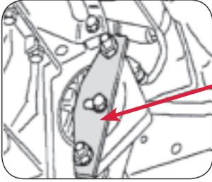
4. Then lock the flywheel using the flywheel locking tool (tool 1).
