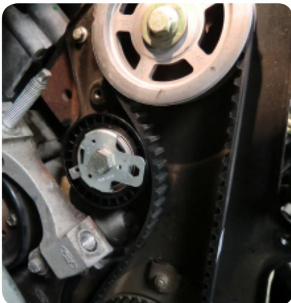
The VKMA 04108 is a very simple looking timing belt kit compared to others that are on the market. It consists of one timing belt (91X20 HSN), one tensioner (VKM 14108) and one set of fitting instructions that are specific to this application.
