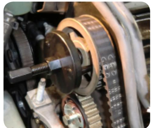
8. Fit the new 'AC' gear (if required) and finger tighten the nut, then back off 1/8th of a turn. **Ensure the gear rotates freely**, as the camshaft gear **MUST** rotate whilst setting the tension. Fit VKM 14108 and finger tighten the retaining nut. Fit the belt, (91x20 HSN) first to the camshaft sprocket and then onto the injection pump gear (the tensioner is last).
