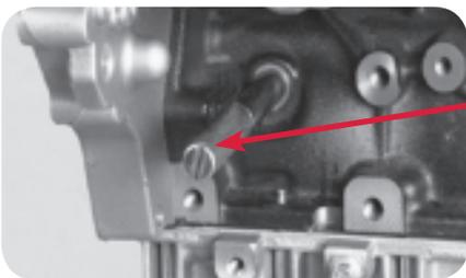
3. Remove the blanking plug from the block and install the TDC timing pin (tool 4).
