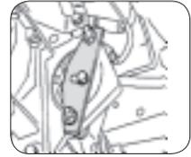
11. Remove all of the locking tools and rotate the engine in a clockwise rotation 6 times.
