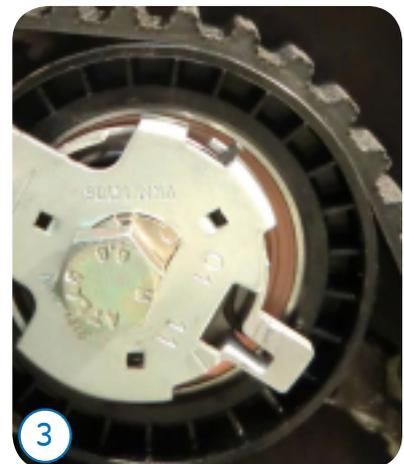
If the tensioner is not set as shown – the technician **MUST** start the procedure again at step **number 9** ensuring that the camshaft gear is loose and the correct procedures are followed.
