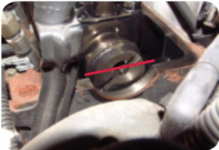
2. Remove the engine cover, turn the crankshaft clockwise and stop just before the TDC on Cylinder #1.
