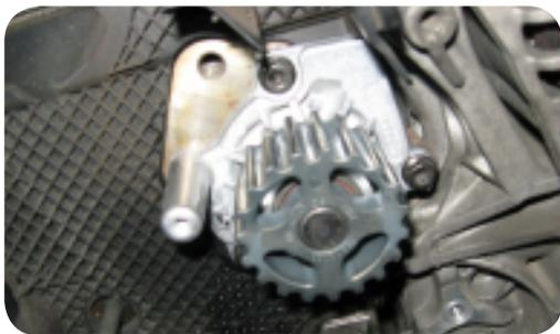
Picture 7: The new water pump fitted.
