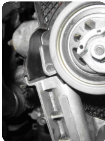
Picture 9: The new hydraulic damper and the tensioner fitted.
