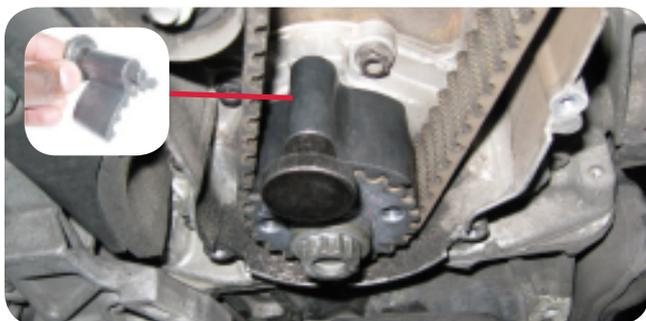
Picture 4: Crankshaft locking tool
