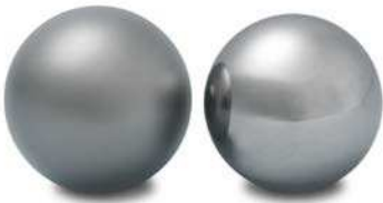
Influence of microcraters due to high frequency current leakage erosion. Comparison between a ball with (left) and without (right) microcraters
