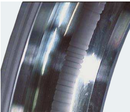
Fluting of the raceways is secondary damage most commonly attributed to the passage of damaging electrical current across the bearing
