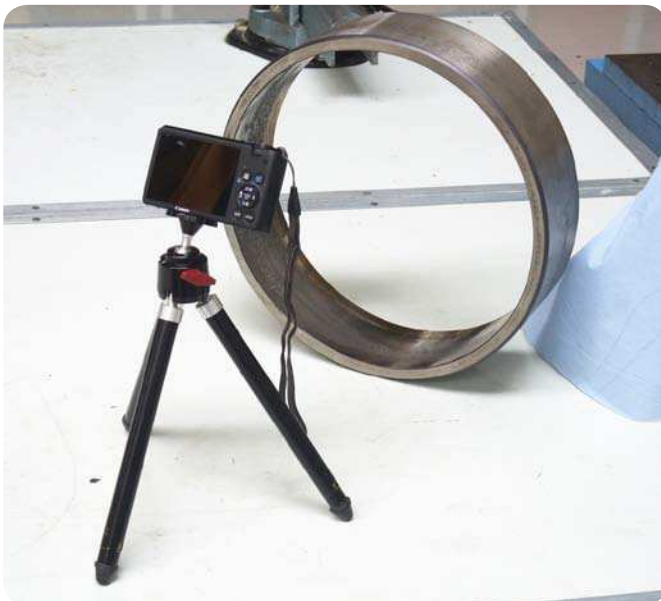
Fig. 12 A compact camera on a tripod is usually good enough to take reasonable photographs of damaged bearings.
