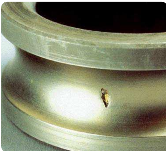
Fig. 3 A small spall (flaking) indicating the end of the bearing life
