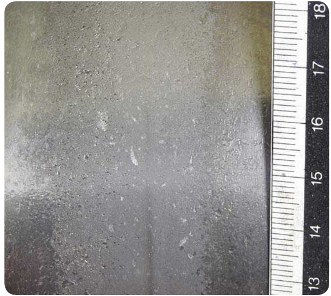
Fig. 13 If there is not enough contrast for your camera to focus properly, use a ruler and focus on the edge that instead.
