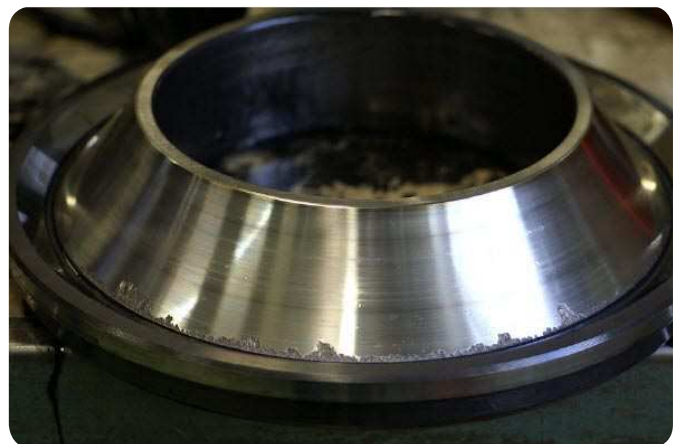
Fig. 2 Bearing made from upgraded steel with spalling
