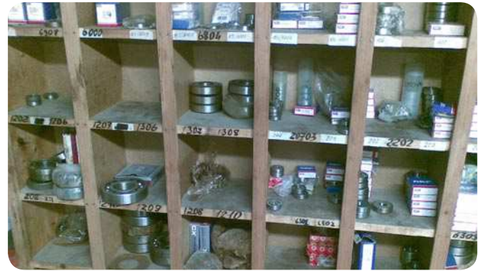
Fig. 1 Bearings, if left unpackaged, collect dust
