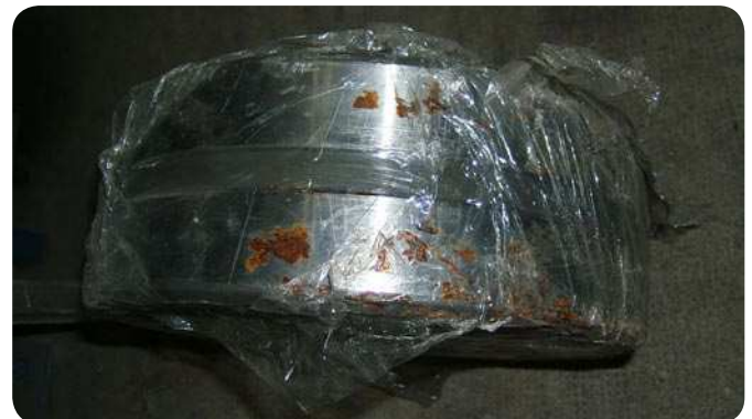
Fig. 3 Bearing, in storage, corroded by humidity.
