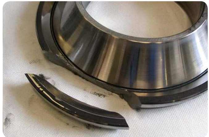
Fig. 1 Bearing with cracked shaft washer
