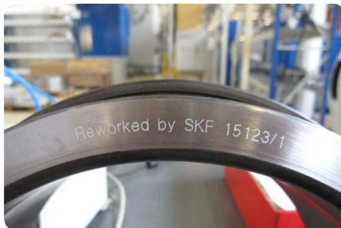
very high speed meaning that the centrifugal forces pushing the rollers against the outer ring are small. The bearing can be put into operation with these remaining corrosion marks.
