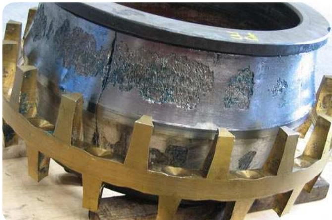
Fig. 6 The corroded inner ring of a deflection compensating roll
