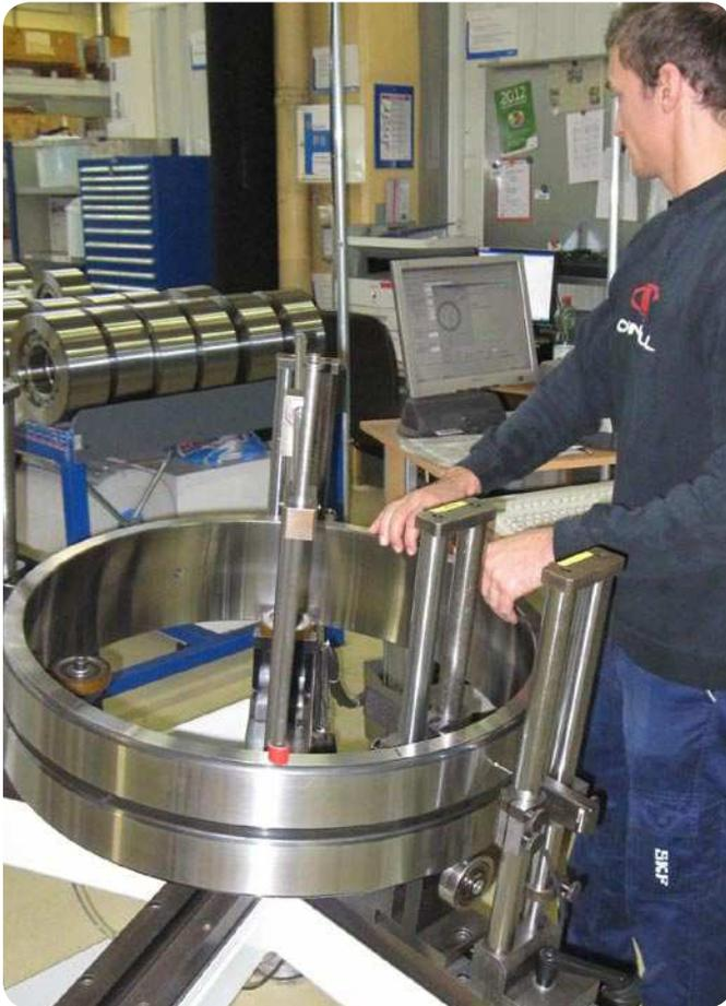
*Fig. 11 Ring ovality and wall thickness variation measurement*
