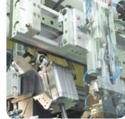
Linear drives for many machine tool axes are equipped with ball screws or roller screws. SKF ball
