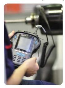
For example, the SKF Spindle Assessment Kit is a complete solution for reliable, simplified, onboard condition monitoring. The kit includes an SKF Microlog Advisor Pro. acceleration sensor, laser tachometer, dial gauge with stand, belt tension gauge and a software package. SKF assists in the set up of measuring points on your machine tool spindles and also offers a consulting service as part of a service agreement.
