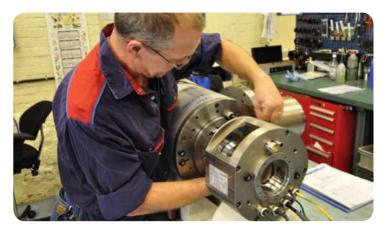
With experienced personnel and critical equipment such as balancing units, precision machining, special measuring tools and advanced vibration equipment, SKF Spindle Service Centres are able to recondition any kind of belt driven and motorized spindle for all spindle brands and designs used in a wide range of applications.
