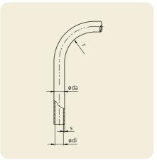
Suitable bending devices can be used to achieve extremely small radii when bending plastic pipes. This requires that the pipe be heated to approx. 150 °C, with a maximum heating time of 20 seconds.
