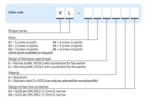
M3 = M10x1 with counterbore for solderless pipe union per DIN 3862 M4 = M14x1.5 with counterbore for solderless pipe union per DIN 3862
