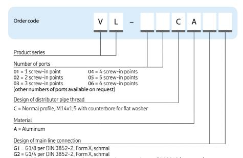
M3 = M10x1 with counterbore for solderless pipe connection per DIN 3862 ( $\boxtimes$  page 14) M4 = M14x1,5 with counterbore for solderless pipe connection per DIN 3862 ( $\boxtimes$  page 14)
