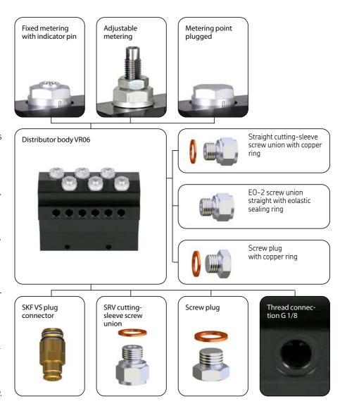
The components made of elastomers inside the single-line distributor are made of FKM (FPM). The distributor body is made from aluminum. The surface is anodized (black color) for long-term protection against corrosion.
