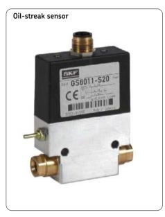
Flow monitors/sensors have the task of monitoring the flow of lubricant from the pump or a piston distributor element to the lube point. Flow monitors with various designs are used for this job. A further task involves monitoring a continuous flow of oil from a pump through a lubrication system. These flow monitors are designed for a throughput ranging from 0,5 cm<sup>3</sup> to 14 000 cm<sup>3</sup>.
