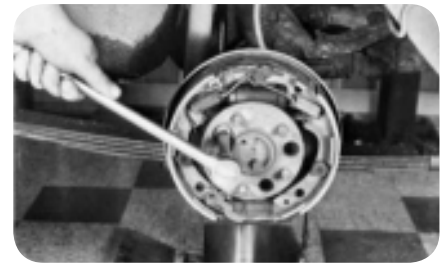
Remove nuts holding retainer plate (fig. 16).
