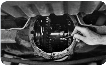
Loosen differential pinion shaft locking bolt (fig. 13).
