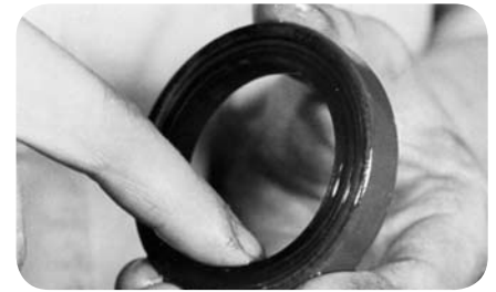
Apply lube to seal lips (fig. 43).
