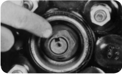
Ford-Turn hub retaining nut to overcome crimp in collar (fig. 23).
