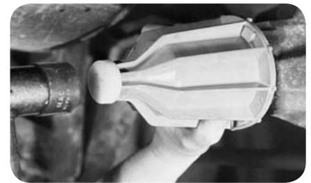
Position installation tool and tap seal into housing (fig. 44).
