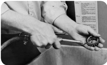
Compressed air may be used to dry cleaned bearing (fig. 6).
