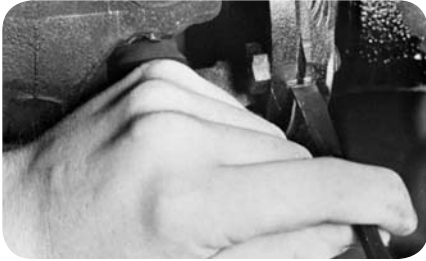
Mark the driveshaft and pinion flange (fig. 39).
