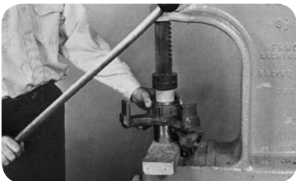
Ford – Use arbor press to install new bearing in hub (fig. 34).
