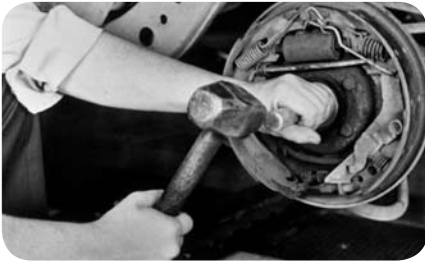
Tap new bearing into shaft cavity (fig. 20).
