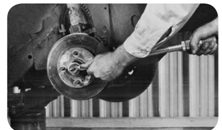
Tighten hub nut while applying brakes (fig. 38).
