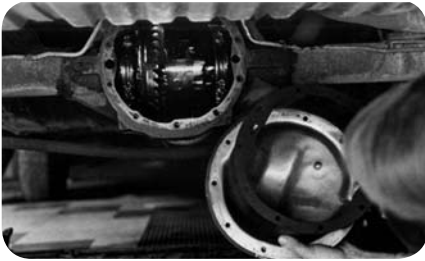
Replace differential cover with new gasket (fig. 21).
