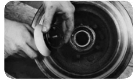
Slide SKF seal onto installation tool (fig. 9).
