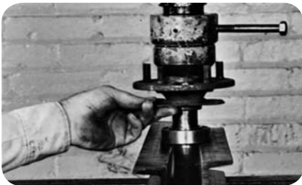
Use arbor press to install bearing (fig. 22).
