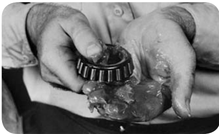
Grease bearing (fig. 7).
