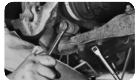
Chrysler – Tighten lower control arm attaching bolt (fig. 36).
