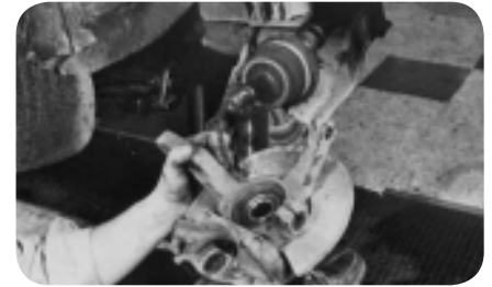
Ford and Chrysler – Place knuckle assembly on ball joint stud (fig. 35).
