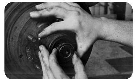
Install outer bearing (fig. 12).
