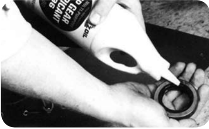
Pre-lube seal with differential lubricant (fig. 19).
