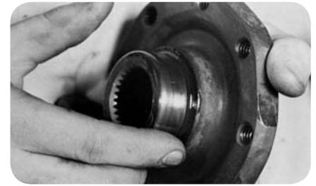
Inspect pinion yoke seal surface (fig. 42).
