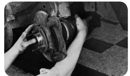
General Motors – Push shaft into hub (fig. 37).
