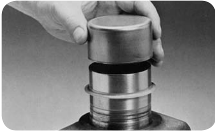
Place Installation tool over Speedi-Sleeve (fig. 46).
