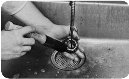
Rinse bearing in clean solvent (fig. 5).
