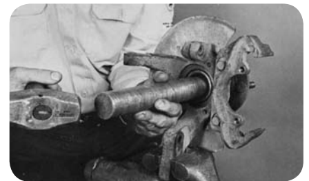
Chrysler – Remove hub from knuckle (fig. 29).
