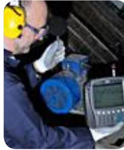
The Microlog Analyzer range includes route-based instruments that work with powerful SKF predictive maintenance software systems and stand-alone instruments that offer on-the-spot advice and signal analysis capabilities. Both options enable you to migrate from time-based to condition-based maintenance, helping you to reduce the risk of unplanned
