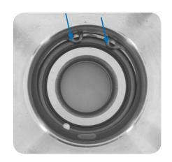
Mount the new bearing into the hub followed by the circlip as per normal HUB 1 assembly technique, including application of the LGAF-3 Antifret paste.
