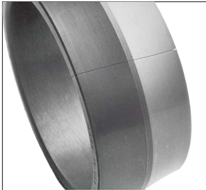
Fig. 16 The fractured inner ring of a spherical roller bearing resulting from excessive drive-up
