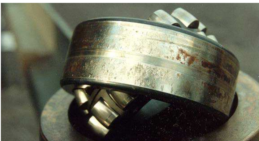
Fig. 8 Fretting corrosion on the bearing outer diameter
