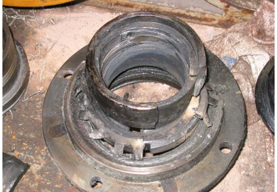
Fig. 11 Part of a bearing inner ring on an adapter sleeve following heavy damage
