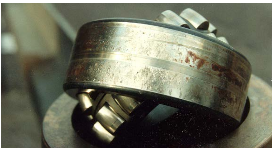
Fig. 8 Fretting corrosion on the bearing outer diameter
