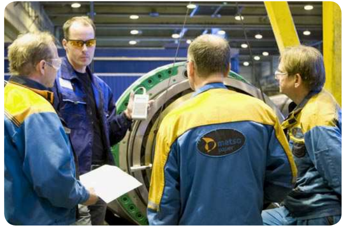
Fig. 3 Eerikki Makinen, SKF Finland's application engineering manager, explaining the CARB toroidal roller bearing mounting procedure with SensorMount
