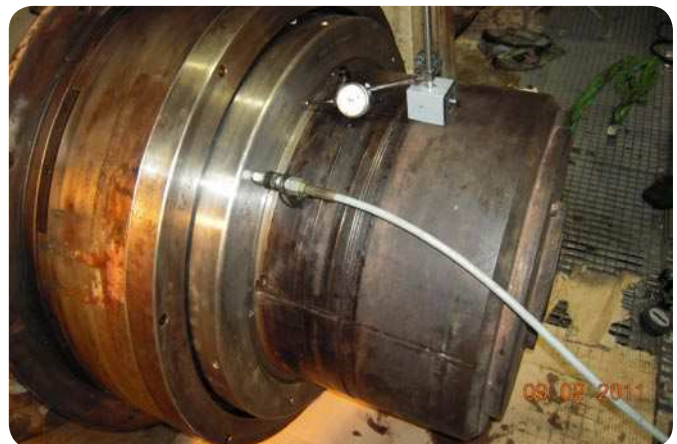
Fig. 1 Axial displacement of the adapter sleeve
