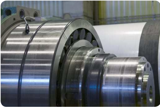
Fig. 6 On the other side, the spherical roller bearing is also equipped to be mounted with SensorMount.
