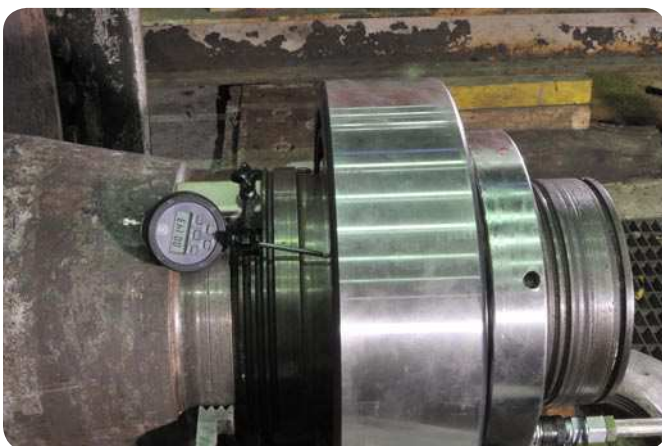
Fig. 17 Dial gauge following inner ring displacement. The dial gauge is supported by a magnetic support fixed on the journal
