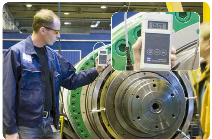
Fig. 5 0.500, the correct interference fit is obtained and the air driven oil pump is switched off.
