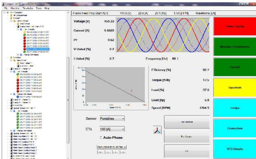
The user interface of the EXP4000 dynamic motor analyzer features an at-a-glance summary of power, motor and machine condition.
