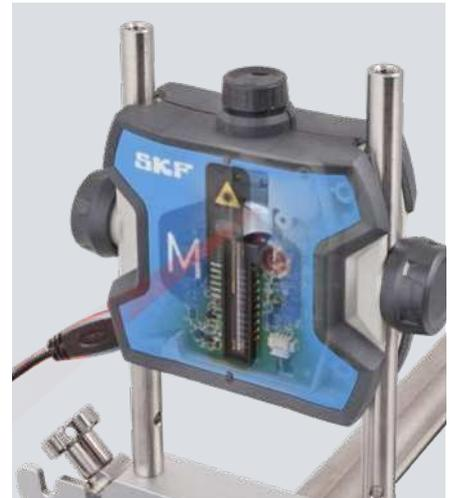
Live view supports intuitive measurements and facilitates horizontal and vertical machine position corrections.
