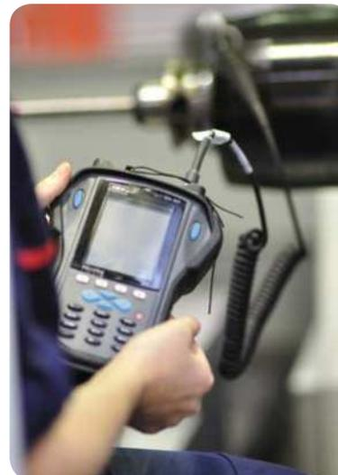
For example, the SKF Spindle Assessment Kit is a complete solution for reliable, simplified, onboard condition monitoring. The kit includes an SKF Microlog Advisor Pro, acceleration sensor, laser tachometer, dial gauge with stand, belt tension gauge and a software package. SKF assists in the set up of measuring points on your machine tool spindles and also offers a consulting service as part of a service agreement.
