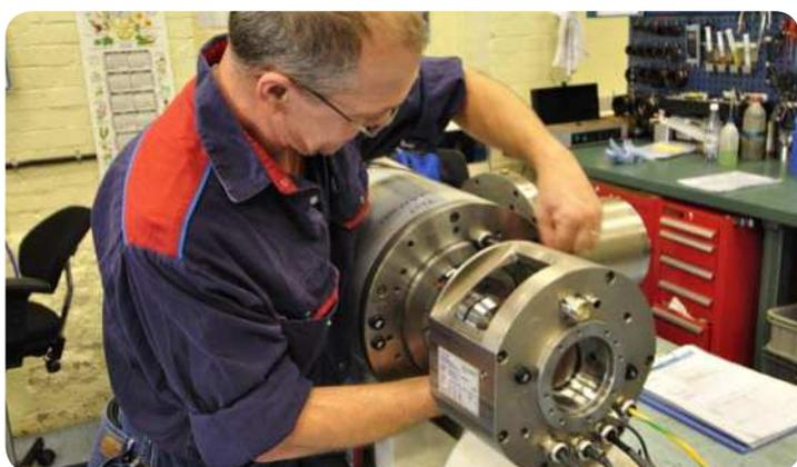
With experienced personnel and critical equipment such as balancing units, precision machining, special measuring tools and advanced vibration equipment, SKF Spindle Service Centres are able to recondition any kind of belt driven and motorized spindle for all spindle brands and designs used in a wide range of applications.
