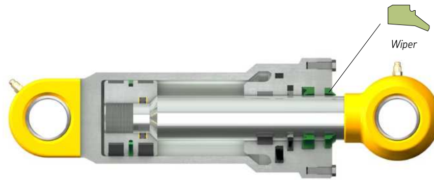
Typical situation for a wiper in a hydraulic cylinder, to protect the internal parts from contamination
