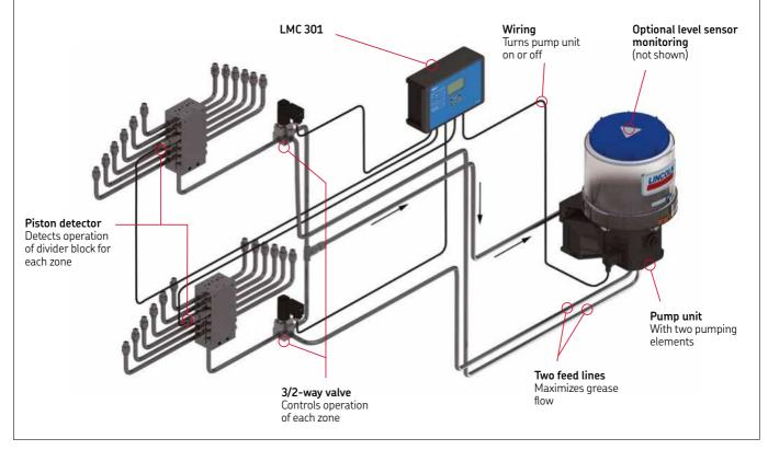
In progressive automatic lubrication systems, a piston pump supplies a defined amount of lubricant through the main line to the metering device that serves each outlet. SKF ProFlex and Lincoln Quicklub systems are designed for specific applications and can be configured to meet the unique requirements of every lubrication point on the equipment.
