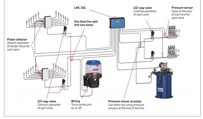
The LMC 301 controller allows for use of up to three pumps, and each pump can operate up to three zones. Each of the pumps can be used with a different system type. Therefore, one unit could operate a single-line system pump and a progressive system pump or a progressive system pump and a dual-line pump.
