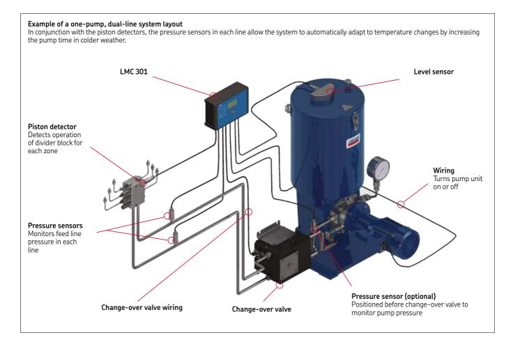
Dual-line lubrication systems, including SKF DuoFlex and Lincoln Helios, utilize two main lines that are supplied alternately with lubricant from a high-pressure pump via a change-over valve, whereby the lubricant also serves as a means of control for the system. These systems are suitable for applications with many lubrication points over long distances in harsh environmental conditions.
