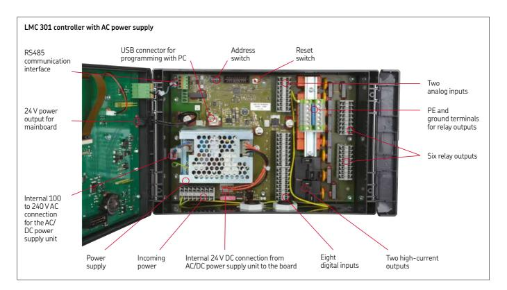
Designed for use with pumps that have no internal controller, the LMC 301 is suitable for applications where sophisticated control and feedback are required. This versatile controller can handle multiple configurations and diverse temperature ranges.
