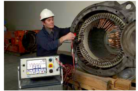
Surge testing a stator is safe with the Baker DX
