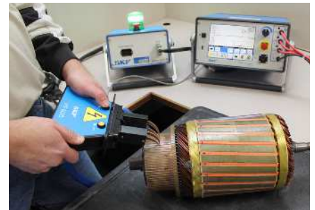
Performing armature tests is easy with the ATF5000 and Baker ZTX low-impedance component test accessories
