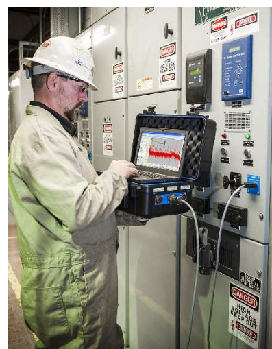
The SKF Dynamic Motor Analyzer - EXP4000 connects easily and safely to an MCC via the EP1000 port mounted on the cabinet door
