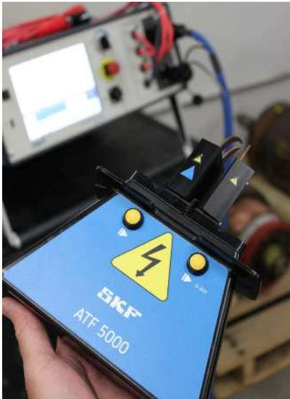
*The SKF ATF5000 accessory works with SKF static motor analyzers to quickly and accurately test traction motor armatures.*
