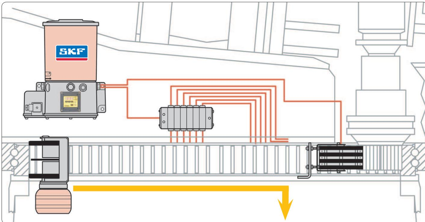
There is a gear wheel with two foam rubber plates on one axle. The intermeshing of the gear wheel and the toothed wheel causes the plates to move simultaneously. These wipes over the toothed wheel continuously remove any excess lubricant from the front sides. The foam rubber plates go through a stripper from where the lubricant is taken to the container that has to be emptied regularly.
