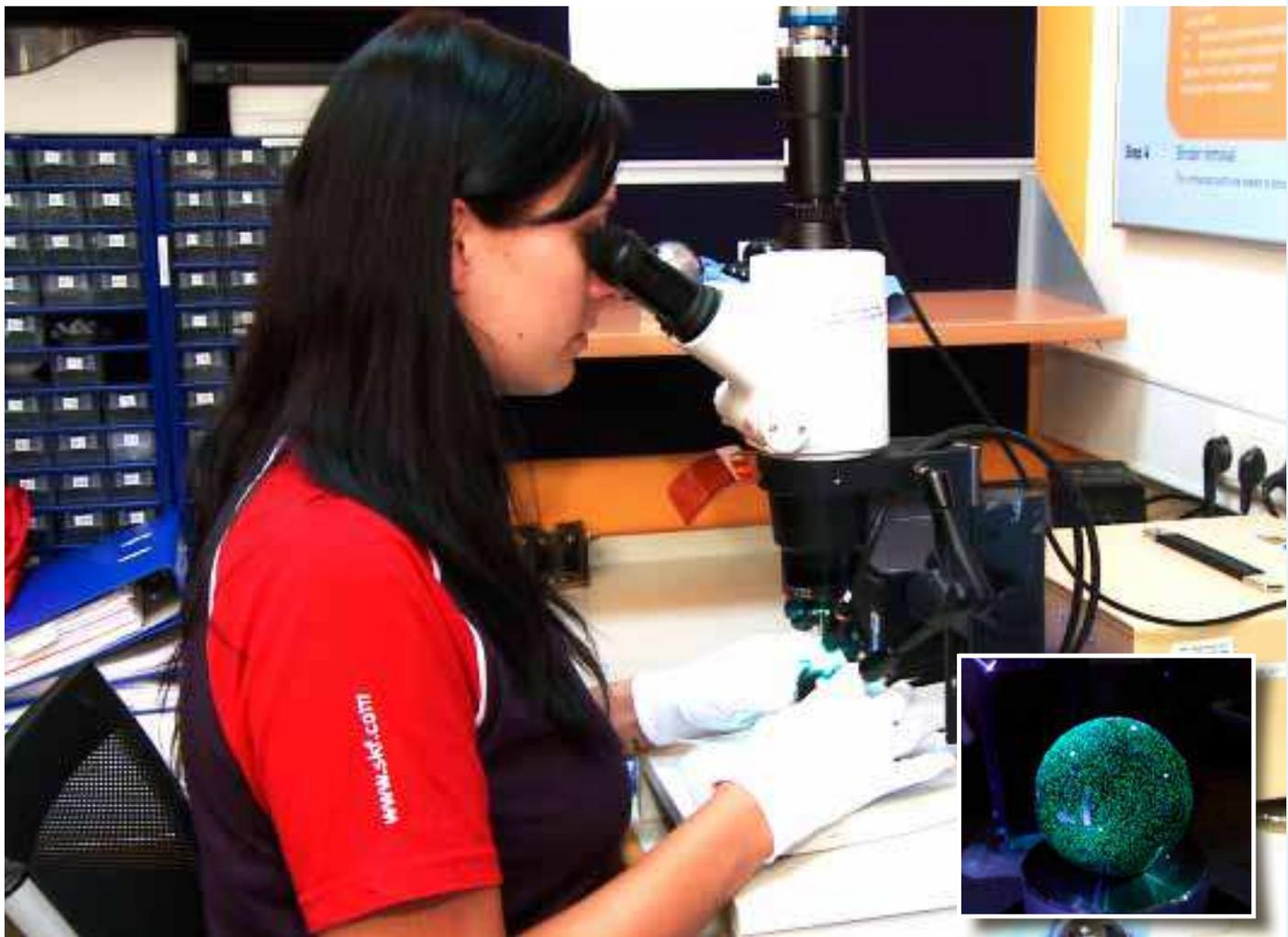
Fig.1: Inspection of 1.875-inch-diameter ceramic balls (right) used for windmill generator bearings.
