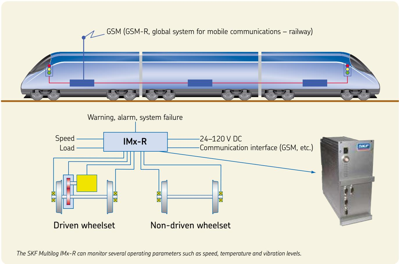
The SKF Multilog IMx-R can monitor several operating parameters such as speed, temperature and vibration levels.
