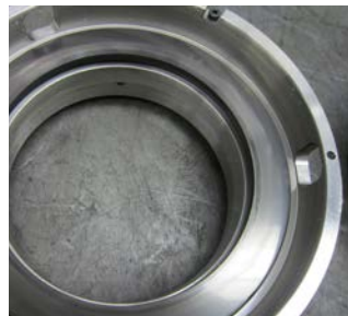
Replacement stationary seal ring ready for re-build and test
