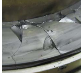
Catastrophic failure of seal face after loss of thrust bearing
