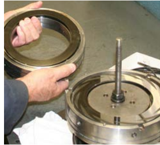
Dry gas seal disassembled for inspection
