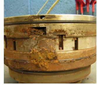
Heavily contaminated dry gas seal from North American refinery
