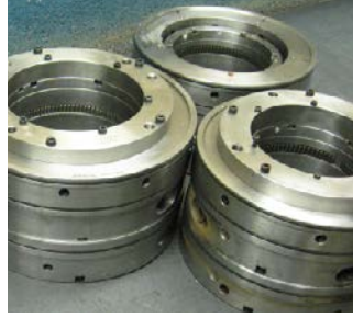
Dry gas seals returned for repair from African methanol plant
