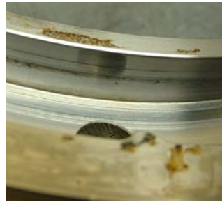
Pitted dynamic O-ring land repaired with nickel plating
