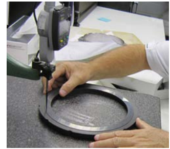
Replacement stationary ring inspected before use in repair
