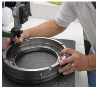
Replacement housing inspected before use in seal repair
