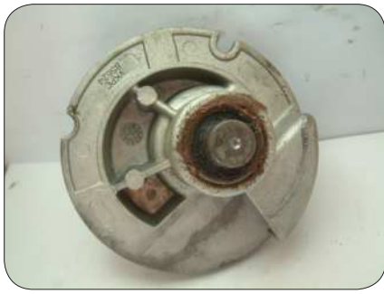
Examples of a damaged water pump:
