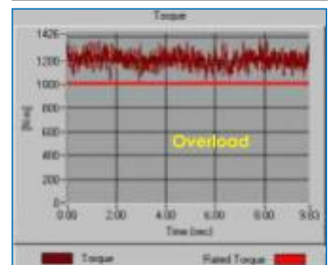
EXP4000 torque signature analysis. Normal torque (top image) compared to a torque overload condition signature (bottom image).
