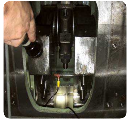
Crank web deflection measurement using an electronic gauge
