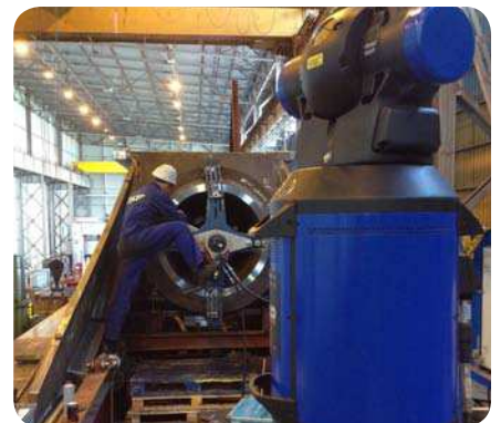
3D measurement in combination with on-site machining
