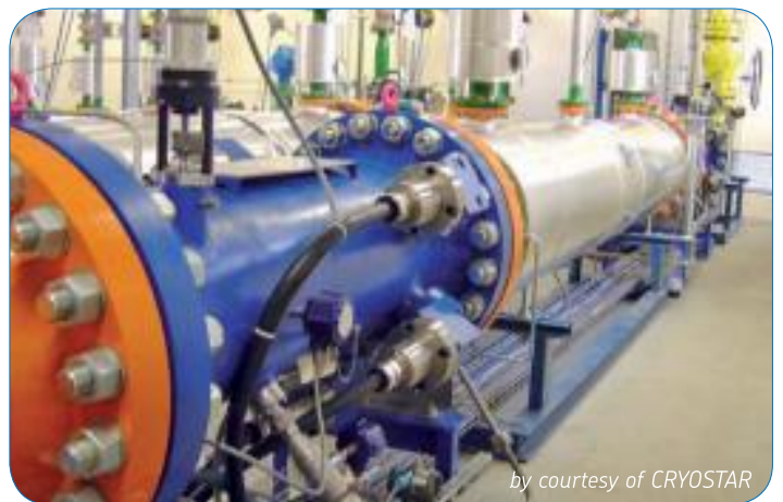
S2M/SKF's very compact electromechanical solution can be located in the pipeline itself.
