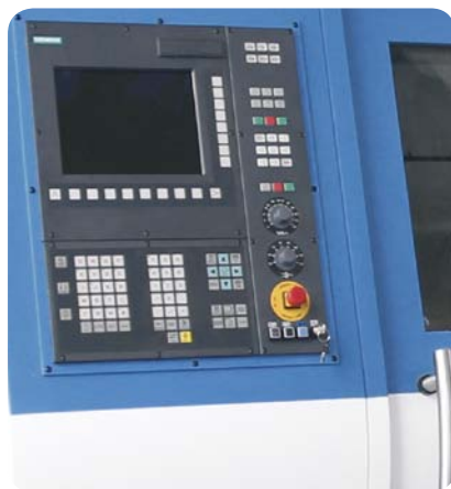
Integrated control unit for the NG 025 machine
