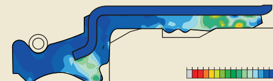
FEA of high pressure valve stem seals Material loading 120 °C and 12 bar pressure
