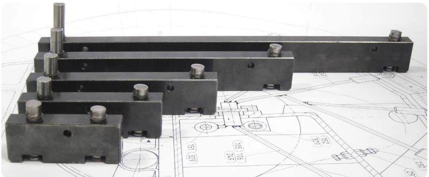
Fig. 1 Five straightedges of various lengths for 1:12 tapers.
