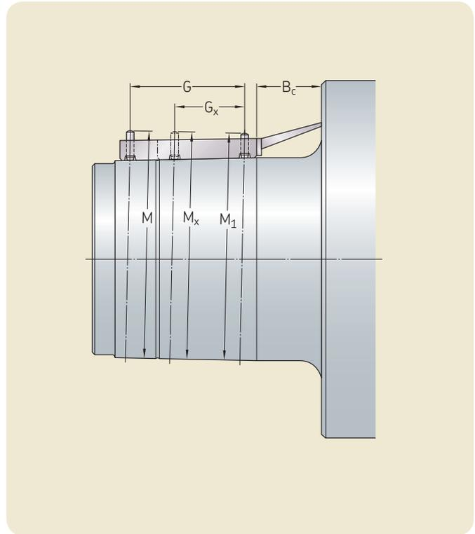
**Fig. 8** Checking straightness with the SKF 9205 taper gauge.
