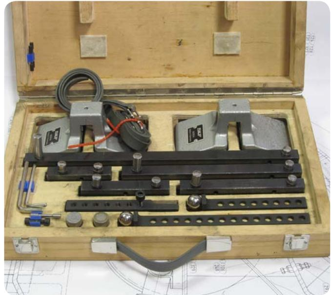
Fig. 4 Complete SKF 920512 taper gauge set.
