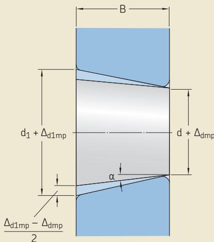
**Fig. 7 Tolerances for 1:30 taper bores.**
