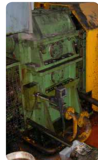
Shown here is the same gearbox, before and after a total refurbishment by SKF gearbox specialists at one of our Gearbox Remanufacturing Centres.
