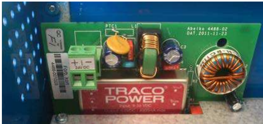
Figure 2 - 2. 24 V DC Power Supply Terminals.
