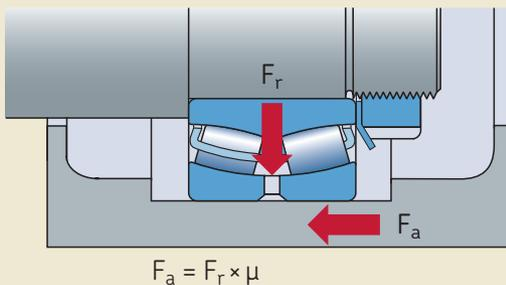
*Uneven load distribution is caused by forces emanating from friction in the axial direction*
