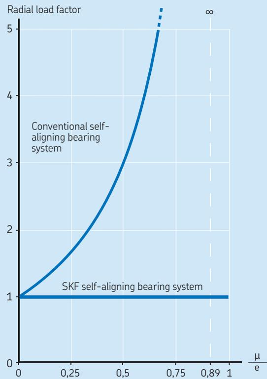
*Required radial load for smooth operation of a conventional self-aligning bearing system with two spherical roller bearings, as a function of housing friction*
