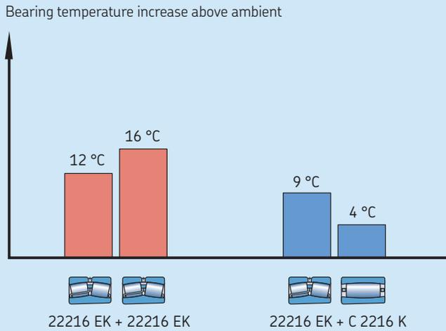
Two other cases of rebuilt industrial fans are shown in **diagrams 4** and **5**. Both examples are conventional centrifugal fans where the spherical roller bearing in the non-locating position was replaced by a CARB toroidal roller bearing of the same size.
