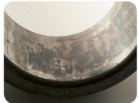
*Through bearing damage analysis, SKF engineers can determine the root cause of bearing failure. Extensive fretting corrosion on this bearing indicates an improper fit on the shaft, which resulted in excessive shaft vibrations and early bearing failure.*
