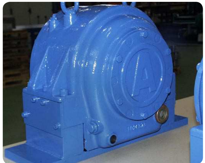
Fig. 14 Rocker housing converted to a fixed housing by SKF.
