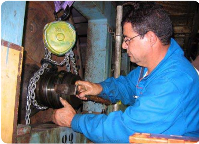
Fig. 2 Checking the contact between bearing and journal with Prussian blue. Note that the hammer is for gently knocking the inner ring to ensure intimate contact.
