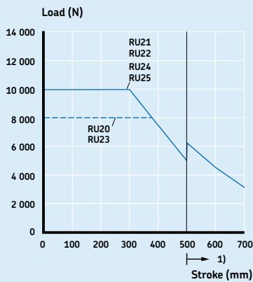
Push load limit, safety factor S=4 (EN 60601 1) retracted length extension at stroke >500 mm
