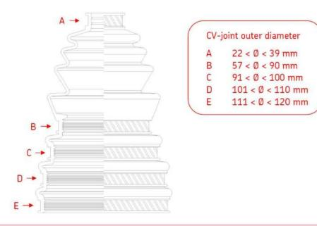
When fitting the universal boot onto the CV-Joint, it is recommended to cut the boot to size after having tightened the clamp.
