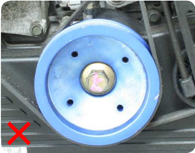
Aftermarket Power Pulleys vs OE Crankshaft Damper
