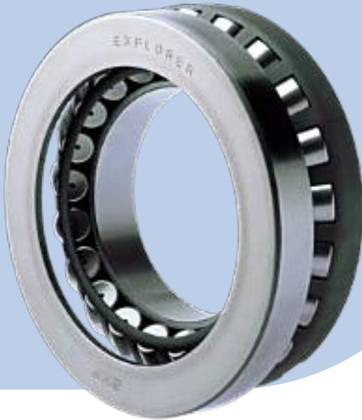
By design, spherical roller thrust bearings are the only bearings that can accommodate substantial radial loads and very heavy thrust loads, making them excellent for combined-load applications. One spherical roller thrust bearing can do the work of a radial bearing and another thrust bearing type, thereby reducing overall bearing arrangement weight, size, and costs.
