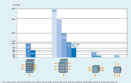
for both outlets are determined by the diameter and the travel of the piston. The selection of the required portion is made during the design of the feeder. A subsequent change of the portions is only possible through a modification of the feeder.
