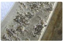
Another form of surface damage is called smearing (adhesive wear). Smearing (skidding) can occur under any of the following conditions:
