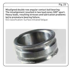
Where two housings supporting the same shaft do not have a common centre line, only self-aligning ball or roller bearings will be able to function without inducing bending moments that otherwise result in shaft deflections and misalignment. Deep groove and angular contact ball bearings as well as cylindrical and tapered roller bearings can accommodate only very small misalignments. Misalignment in these bearings typically causes edge loading, which can result in premature fatigue.
