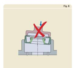
When installing a seal into a housing bore:
