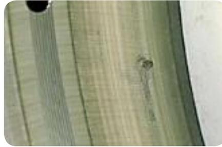
**Surface initiated fatigue in the outer ring of a spherical roller bearing.**
