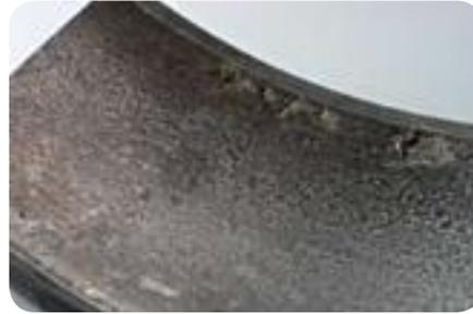
**TBU outer ring with heavy indentation damage**
