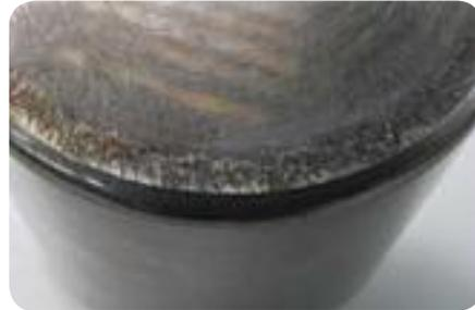
*Smearing on the large diameter thrust face of a tapered roller*
