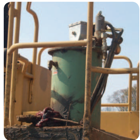
Over-filled reservoir with no overflow prevention system
