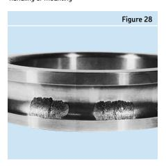
Smearing caused by excessive force in mounting
