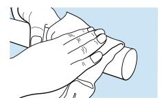
Step 1c Lubricate the shaft with a light oil.
