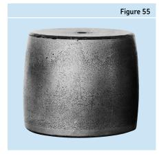
Corrosion on roller surface caused by water in lubricant while bearing was standing still
