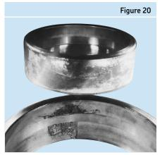
Fatigue from chip in housing bore
