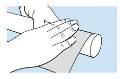
Step 1b Wipe shaft with clean cloth and check the
