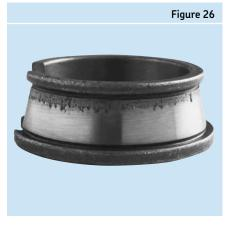
Advanced spalling caused by edge-loading
