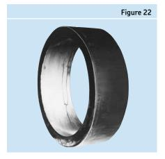
Mirror view shows how raceway is affected by out-of-round housing
