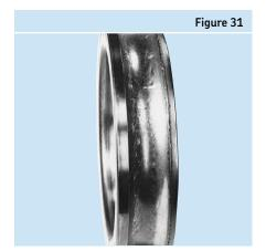
Electric pitting on surface of spherical outer raceway caused by passage of relatively large current
