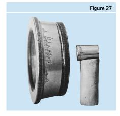
Fatigue caused by impact damage during handling or mounting
