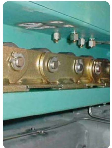
Contact-free oil lubrication with PMA2-nozzles in a paint shop
