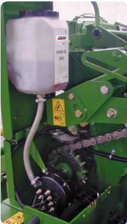
Agricultural machine (baler) with MOS/MOP 212 lubrication system
