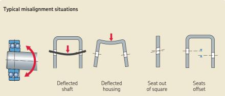
Self-aligning ball bearings accommodate up to 3 degrees of misalignment without increasing friction and frictional heat
